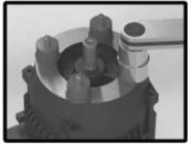
Remove old motor mounts and replace with new motor mounts. Tighten mounts to 8Nm.
