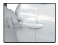
Fit oil return tube and position tube to drain oil back to machine enclosure, sump or collection vessel.
