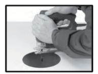
Cut extraction hole in machine enclosure.
